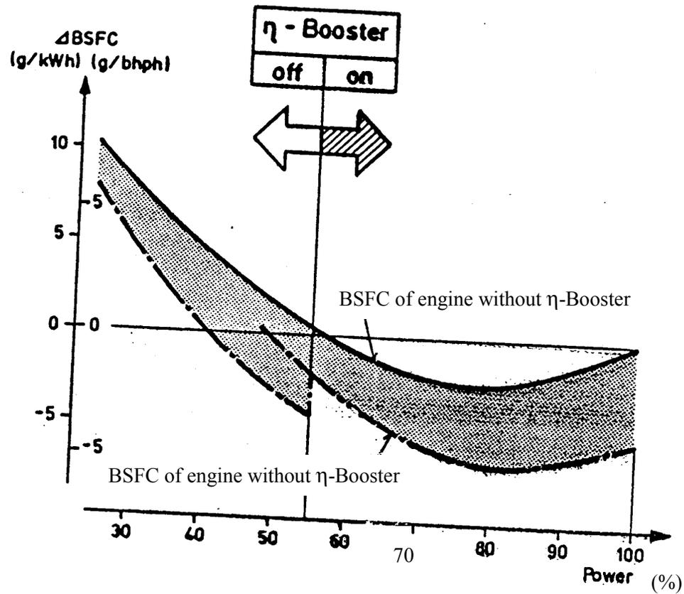
**Figure 3.4** Effect of efficiency-booster on the BSFC of a typical marine slow speed engine
