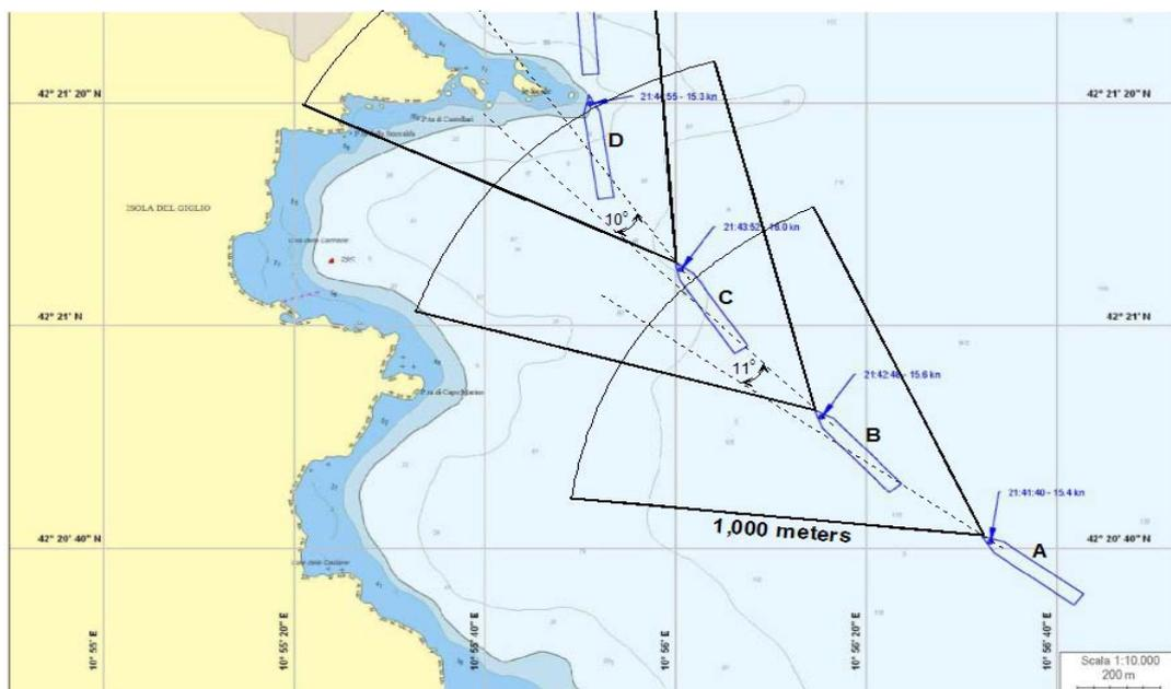
**Figure 4: Ground Track of Costa Concordia, Annotated with Coverage for Forward-Looking Sonar Navigation**
