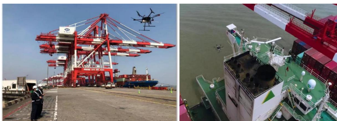
Figure 12- Preliminary positioning measurements of ship plume by UAV
