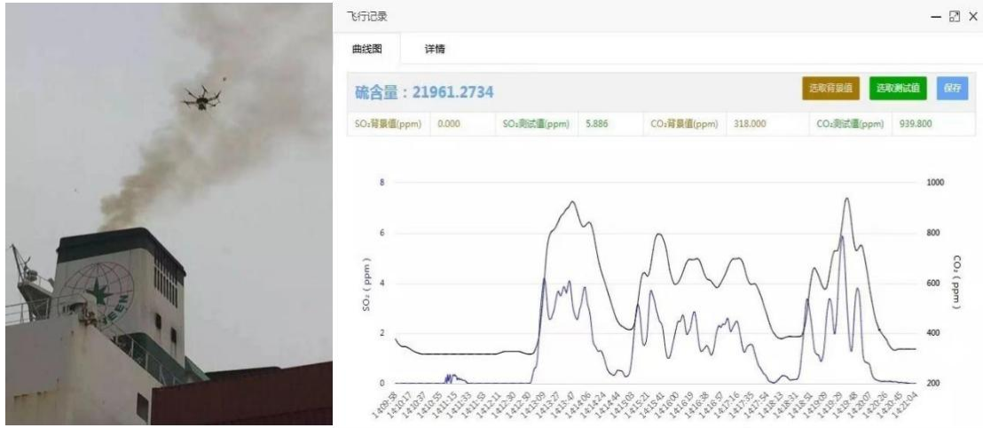
Figure 13- Drone close to the ship exhaust funnel for exhaust gas collection and inspection
