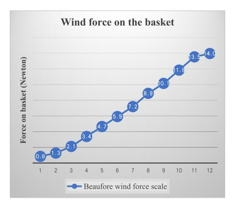
**Figure 27** shows the effect of wind (from force one to force twelve) on the basket, ranging from 0.8 Newtons to 14 Newtons. While one magnet provides 4415.5 Newtons (450kg\*9.81N/kg) of holding force (**Figure 28**), this is obviously more than 14.0 Newtons. This means that the basket will not roll and twist under this situation.
