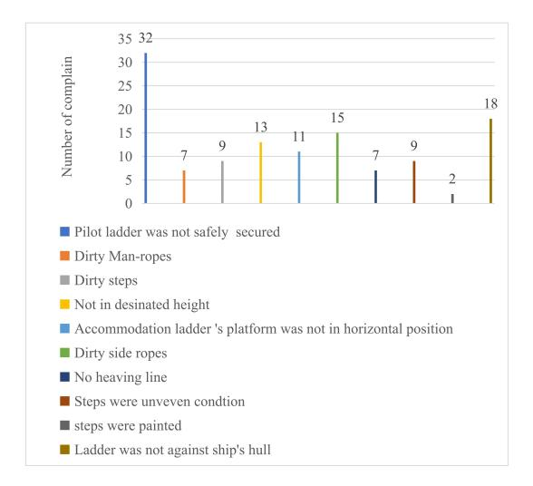
**Figure 21** shows the non-compliances of the pilot ladder that were complained about by pilots. According to the feedback from the 123 respondents, the non-compliances items that were complained about are as indicated:
