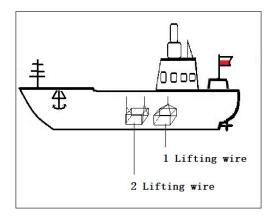
The use of two wires means that there are two points of force which, together with the contact point between the wheel and the hull, form three points of force, making the movement of the lift basket more stable, whereas a single wire does not have this effect.
