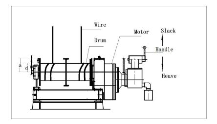
The drum is a split drum for two wire ropes, and the length is sufficient for the wires to be fully wound in effective working length. When deciding the length of the drum, the rope size (diameter), vessel size (moulded depth) and installation position should be taken into consideration.
