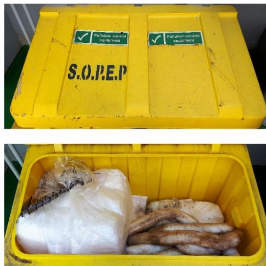
Figure 9. An example of sorbent materials equipped in a Shipboard Oil Pollution Emergency Plan (SOPEP) (Vuong, 2019b)
