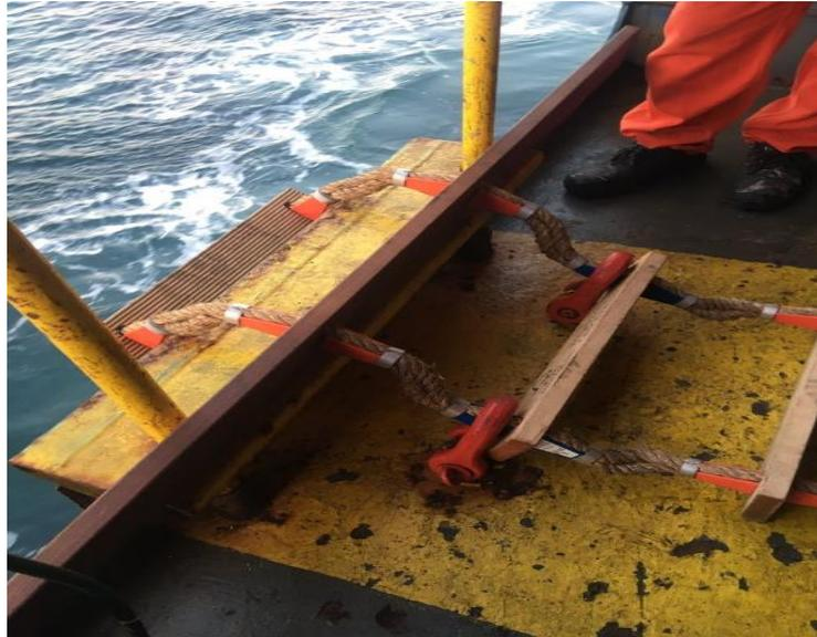
*Figure 4 Faulty ladder, risks of ladder slippage when exerting weight*
