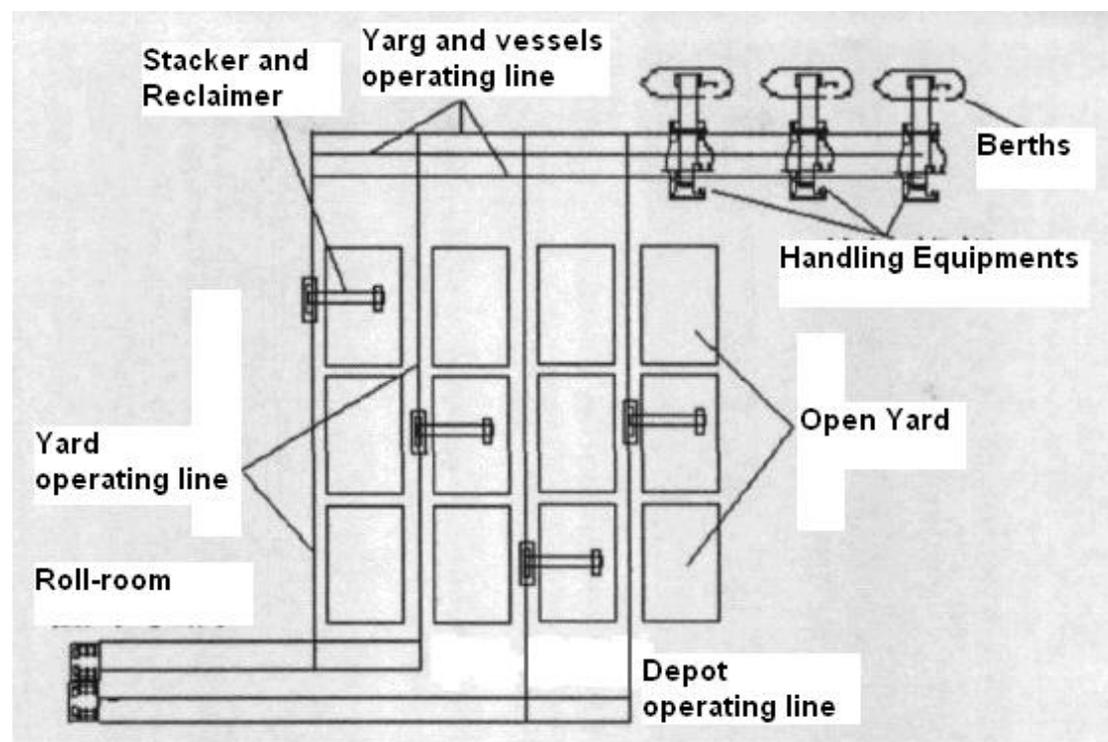
Berth is the term used in ports and harbors to define a specific location where a vessel may be berthed, usually for the purposes of loading and unloading. Most berths will be alongside a quay or a jetty (large ports) or pontoons (small harbors and marinas). Berths are either general or specific to the types of vessel that use them in the process. The size of the berths varies from 5-10m for a small boat in a marina to over 400m for the largest tankers.
