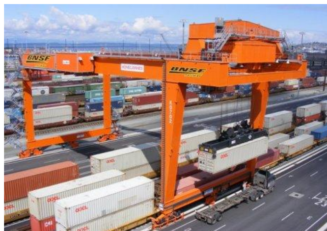
Figure 4.17. Wide span of RMGC
