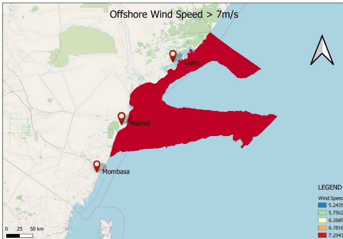
Figure 6.1 2 A map showing areas with Kenya's mean offshore wind speeds of > 7 m/s. Created using QGIS (Author, 2021).
