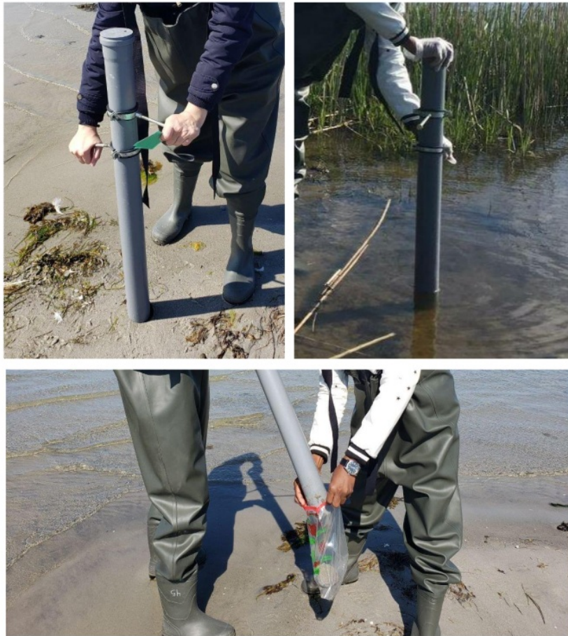
Figure 4: Collecting sediments from sites using a core sampler
