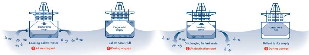
Figure 1. Schematic diagram of ship's ballast water loading and discharging. (Source: IMO, n.d.)
