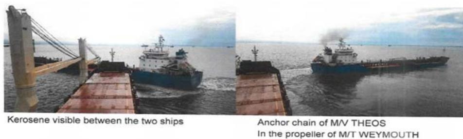
**Figure 4. 8:** *M/T Weymouth* and *M/V Teos* after the collision
