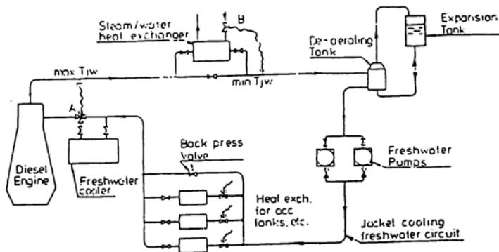
**Fig. 2. 9 Jacket cooling water heat energy recovery**
