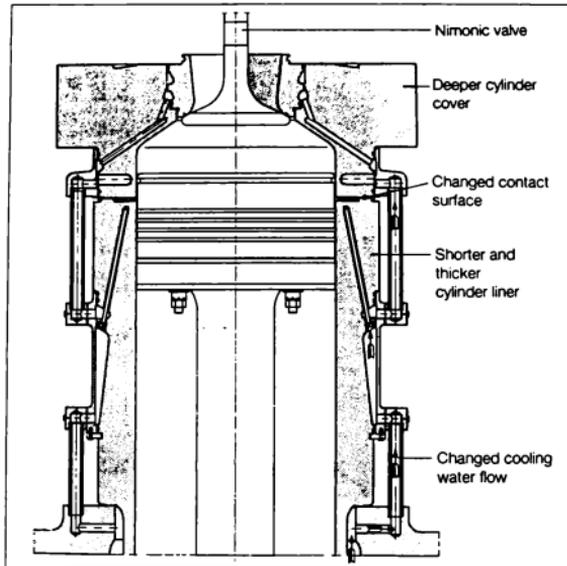
**Fig. 2. 10** *The new combustion chamber design*
