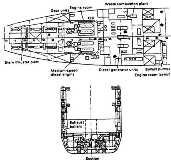
**Fig. 2.3 Medium-speed diesel machinery arrangement**
