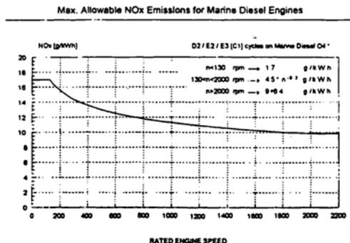
**Fig. 3.6 Proposed IMO emission limits**
