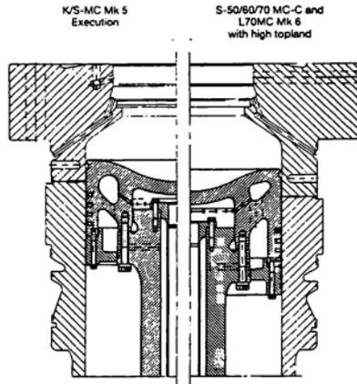
**Fig. 2. 5 Piston / ring pack assembly MC vs MC-C**
