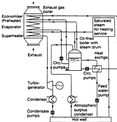
**Fig. 2. 7 Single pressure boiler turbo-generator system**
