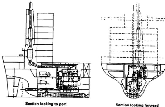
**Fig. 2. 2 Slow-speed diesel machinery arrangement**
