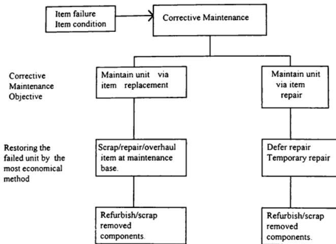
Figure 5.2 Alternative corrective maintenance actions for a complex replaceable item.
