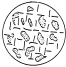
Corrosion in a salt-water droplet on steel just after the droplet has been attached
