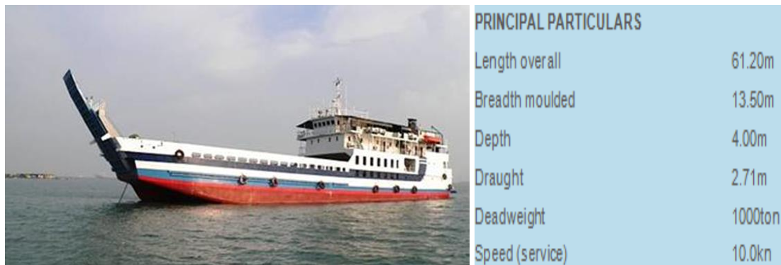
Figure 10: An image of a feeder vessel with its particulars
