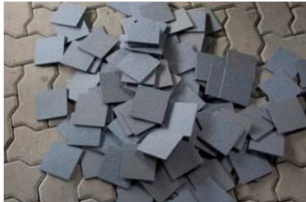
Figure 1: Biodegradable wood-based oil binders (BioBinders) Source: Rostock University
