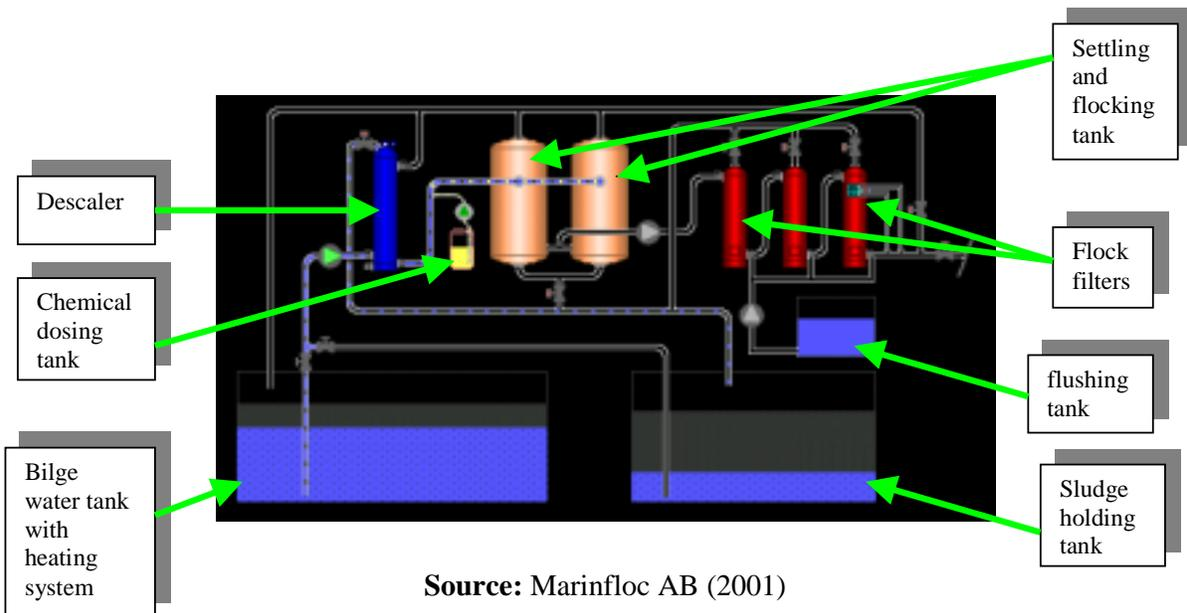
in the bilge water tank and then fed to the oil descaler where all free oil is separated (see figure 8). The oil sensor, after sensing oil, activates the oil release valve to drain
