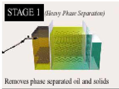
Figure 9 (a): Biomechanical oily water separator ,stage 1
