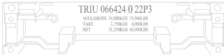
Figure 28 - Schematic Diagram of Flat Rack Permissible Payload (Examples)
