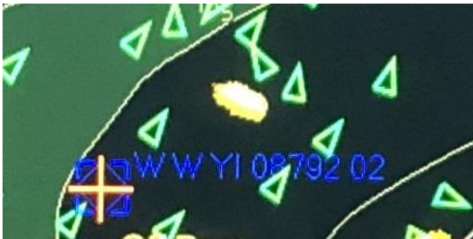
Figure 11 – A selected AIS FNL target displayed as a blue solid diamond in broken squares Source: Dalian: Author.
