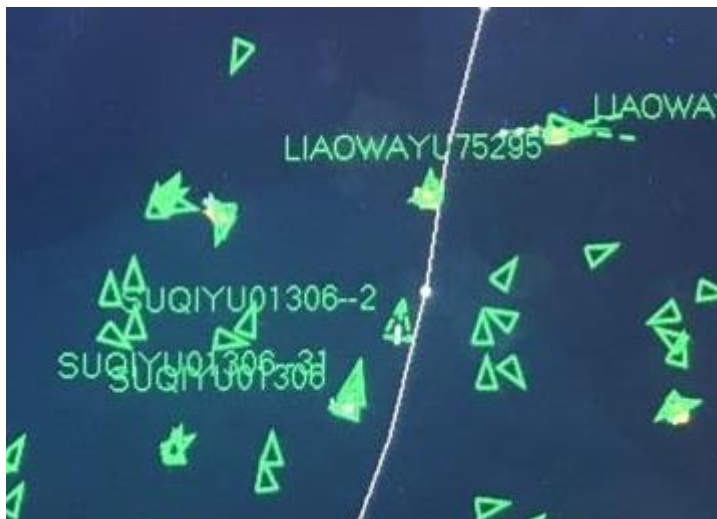
Figure 9 – A screenshot of radar of green triangles shown by AIS FNLs Source: Dalian: Author.
