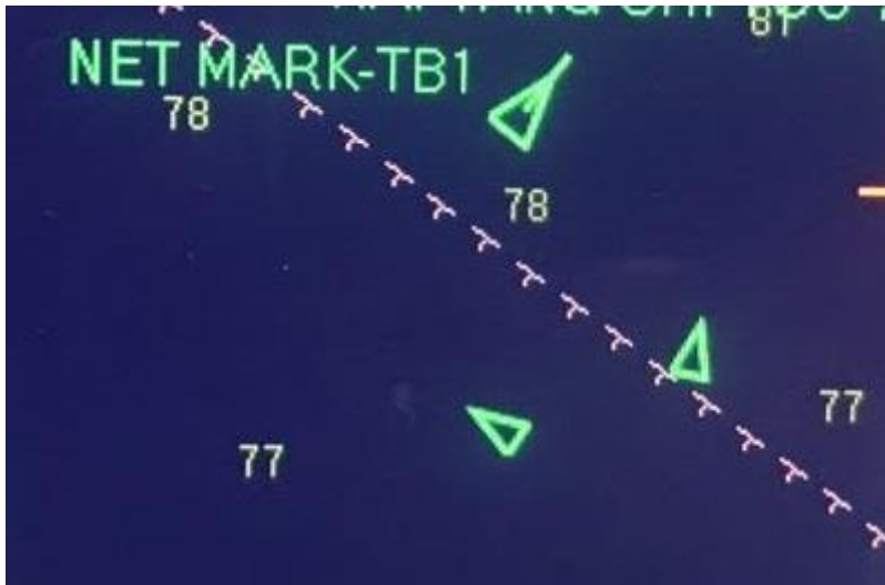
Figure 10 – A screenshot of radar of AIS FNLs in green triangles with their name “NET MARK”
