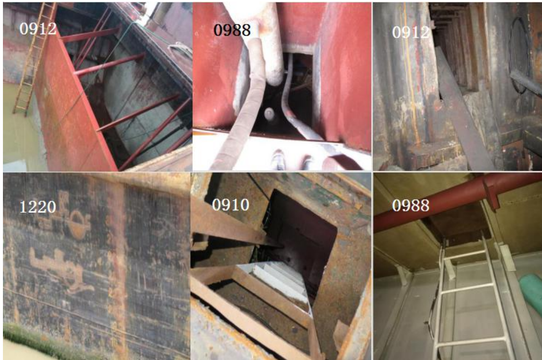
Figure 5.2 – Illegal reconstruction of sand carriers Source: Photos taken by the author during FSC inspection
