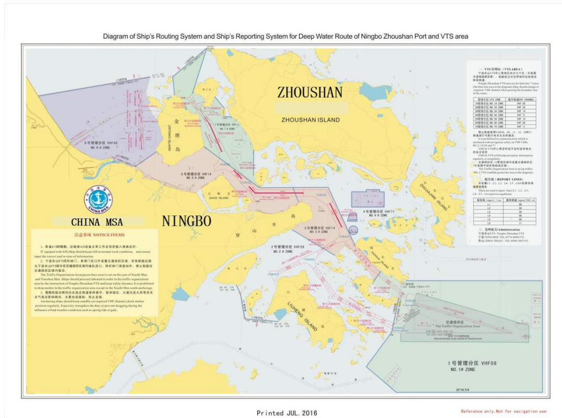
Figure 4.1 - Schematic diagram of ship routing and reporting system of Ningbo-Zhoushan Port Source: Ningbo MSA.
