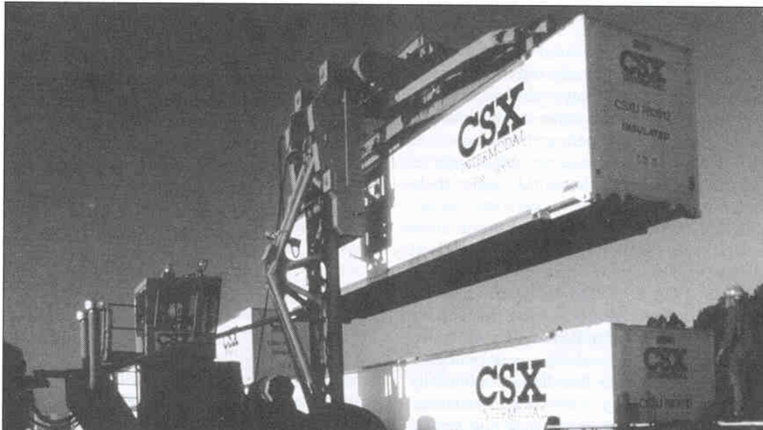
Exhibit 7. Container handler loading container on doublestack railcar.
