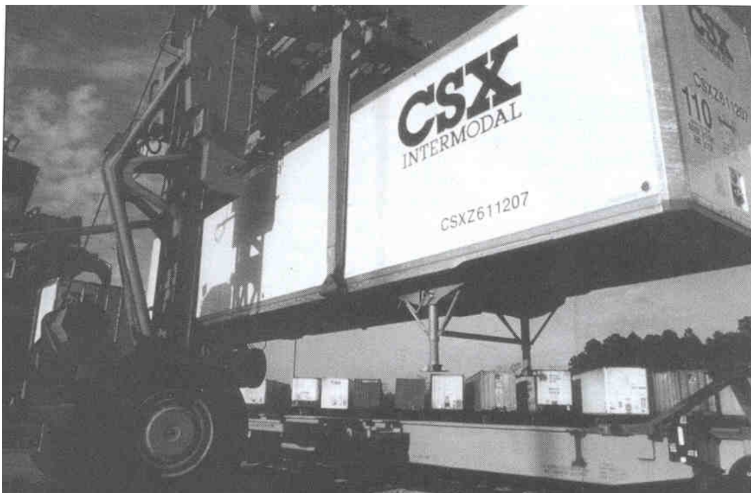
Exhibit 8. Trailer handler loading a trailer on to a rail flatcar.
