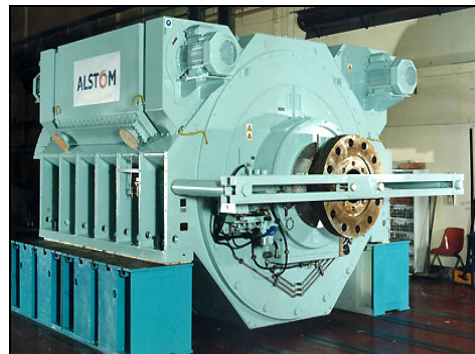
Figure 30: ALSTOM 20MW motor
