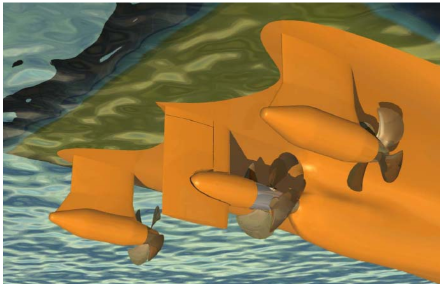
Figure 42: Hybrid propulsion for ULCS (Source Wärtsilä)
