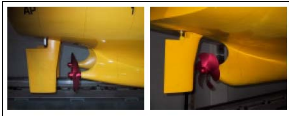
Figure 39: Difference between twin and single screw arrangement (Source: MARIN).
