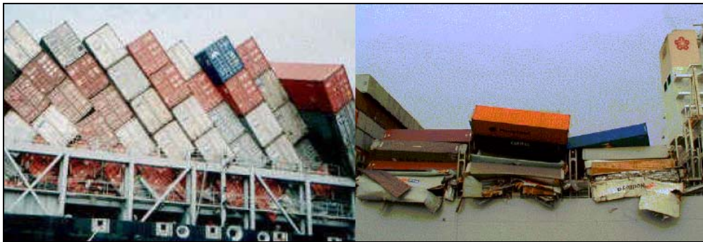
Figure 45: Damages to containerships due to parametric rolling
