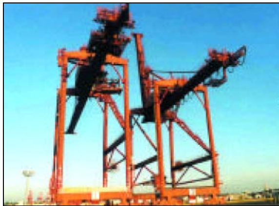
Figure 52: Modification of Gantry crane capacity (Panamax to Post - Panamax)
