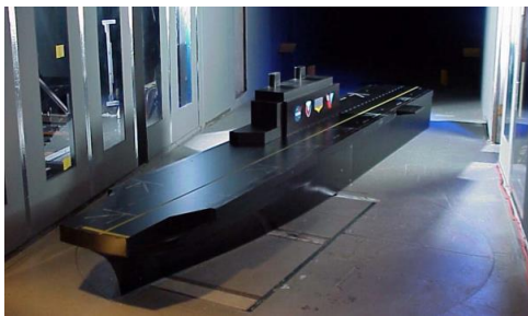
(a) 1:48 LHA physical model in wind tunnel
