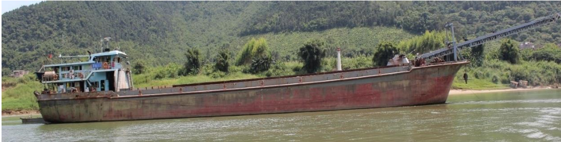
Figure 3.3 – A Typical inland self-unload carrier in the PRD
