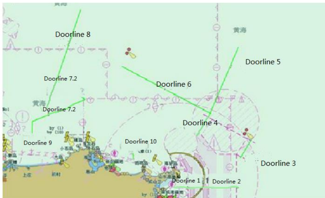
Fig 2.2 The Gate-line of Chengshanjiao water area TSS schematic diagram
