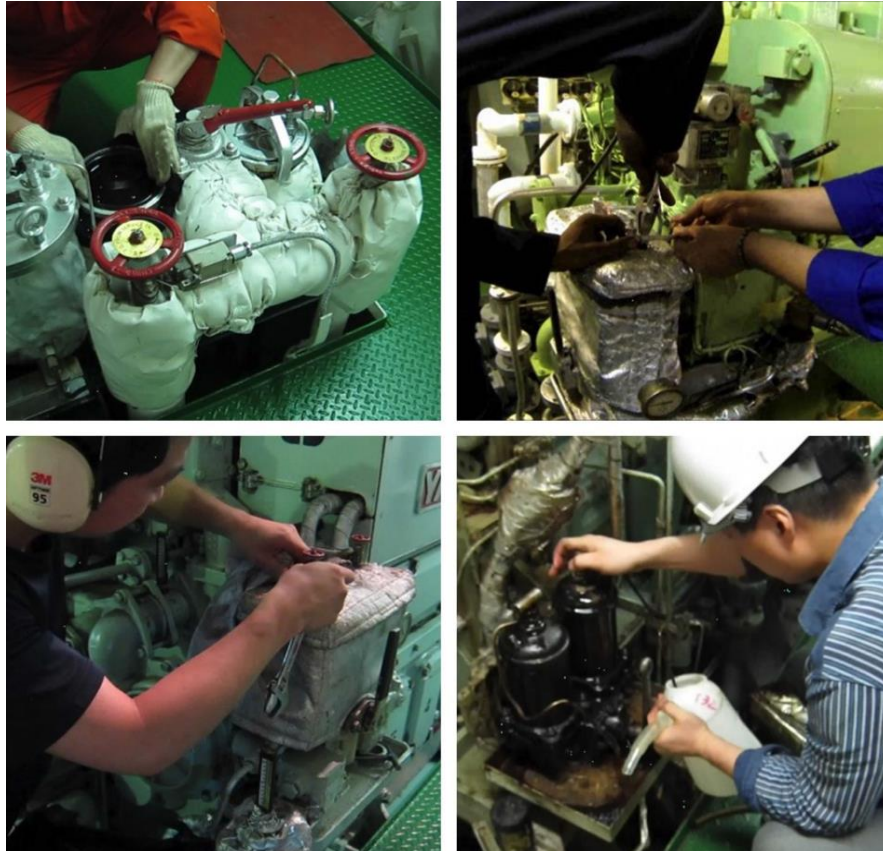
Figure 3.1 - Sampling in Final Filter
