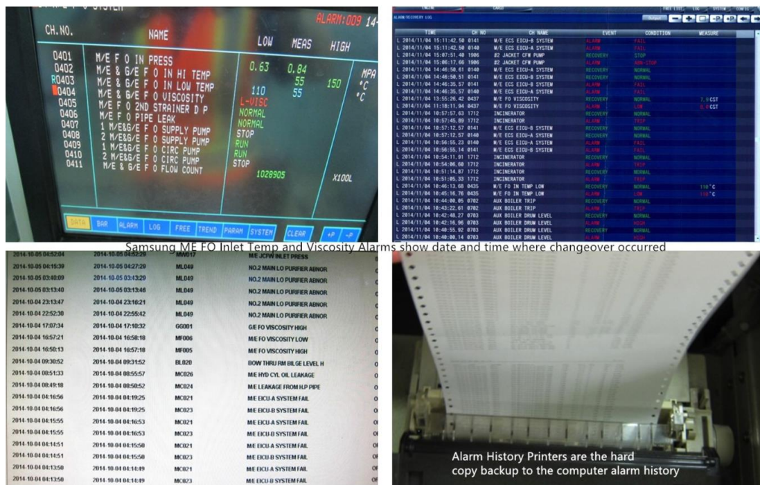
Figure 3.4 - Fuel temperature and viscosity alarm
