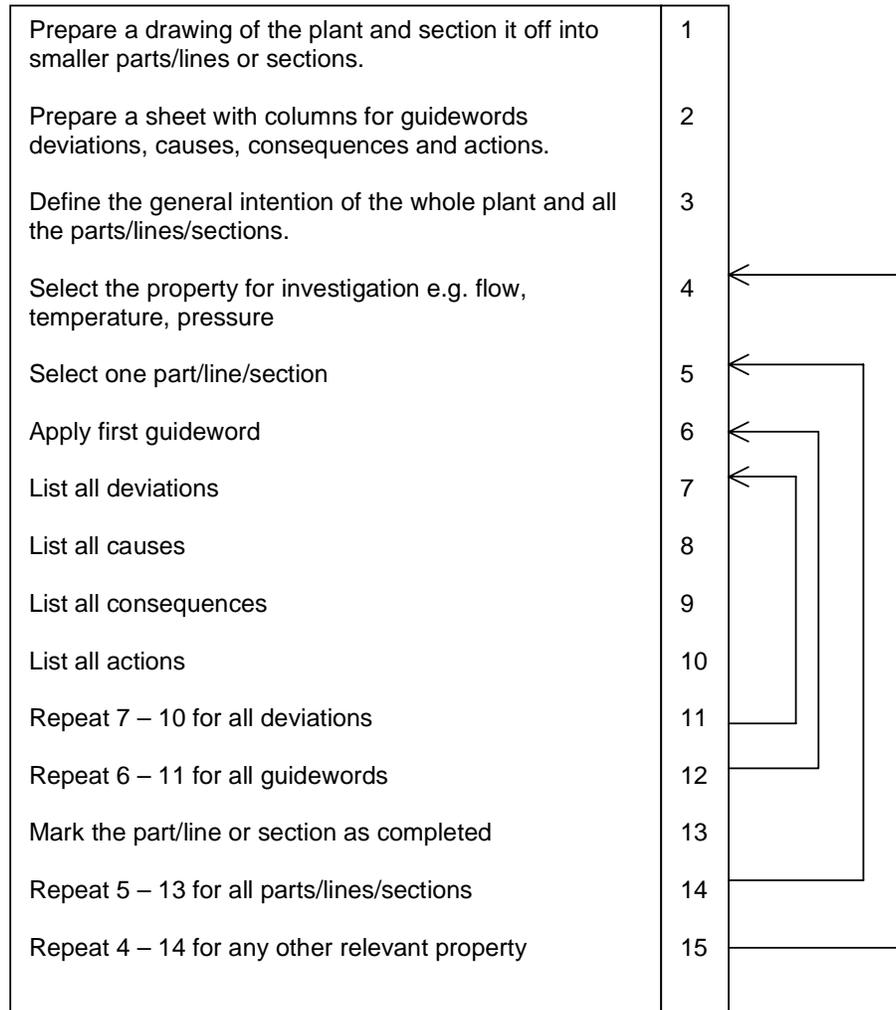
Figure 4.1: Process of Hazard and Operability Analysis
