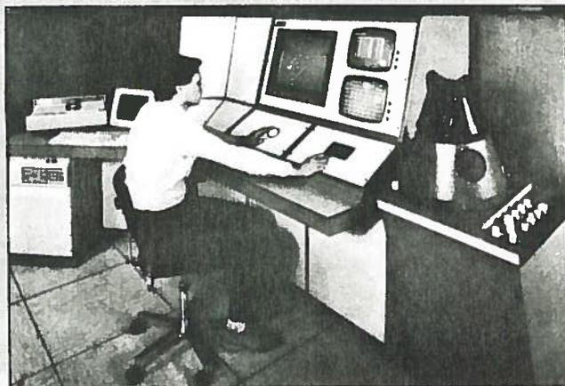
The redesigned instructor's console features a Labelled Plan Graphics Display (LPGD) similar to that used with naval equipment. A conventional radar display is also available.
