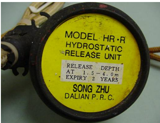
Figure 1.4 - Not approved device. Source: AMSA.
