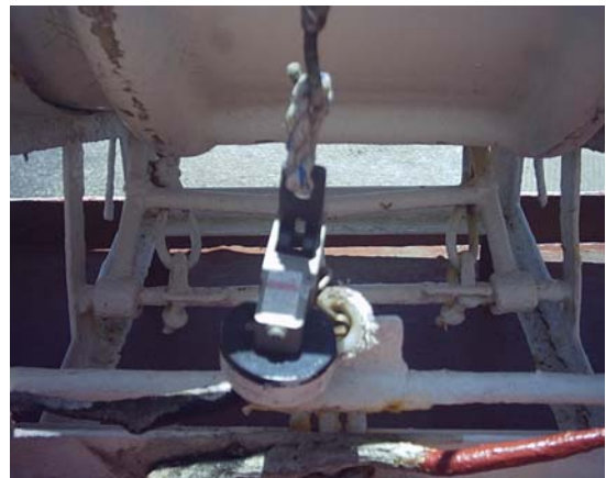
Painter not connected to the HRU.
