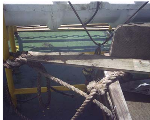
Manual launching obstructed.
