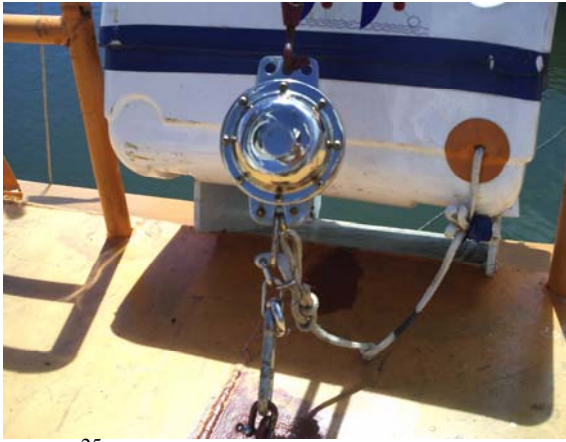
HRU 25 installed upside down.
