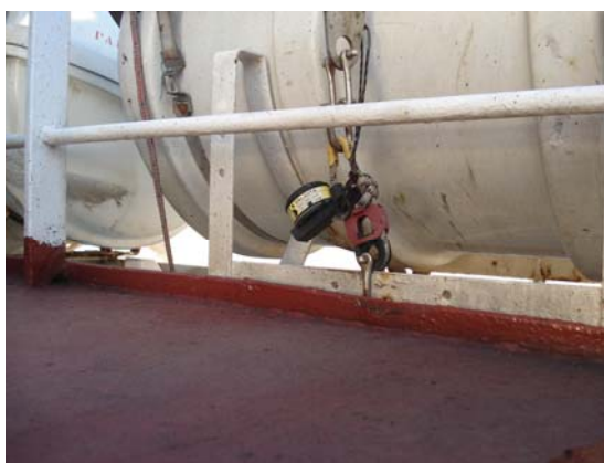
Painter not connected to the weak link.
