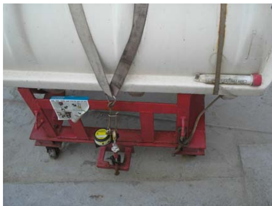
Figure 3.8 - HRU incorrectly installed.
