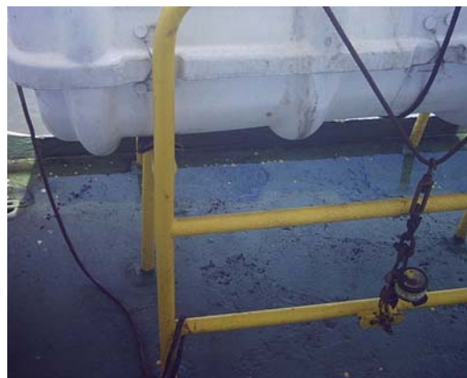
Painter connected to a fix point.
