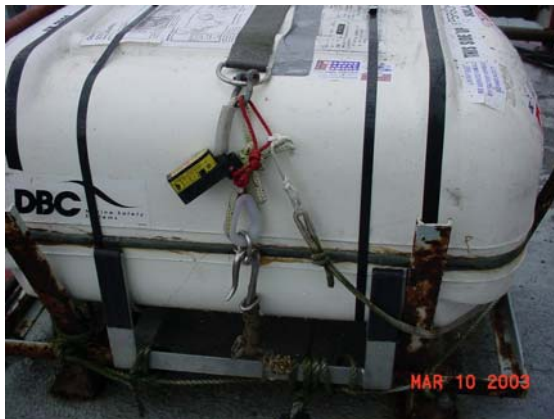
Painter and hook incorrectly connected.
