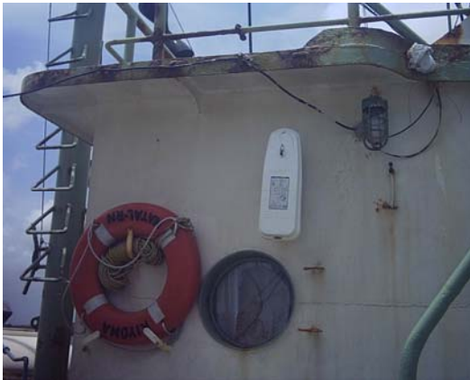
Obstruction to free-flotation.
