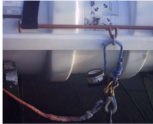
Manipulated and incorrectly set HRU.
