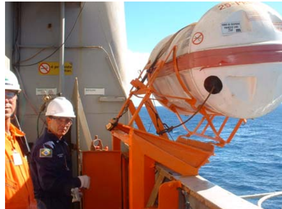
Painter connected to the cradle.
