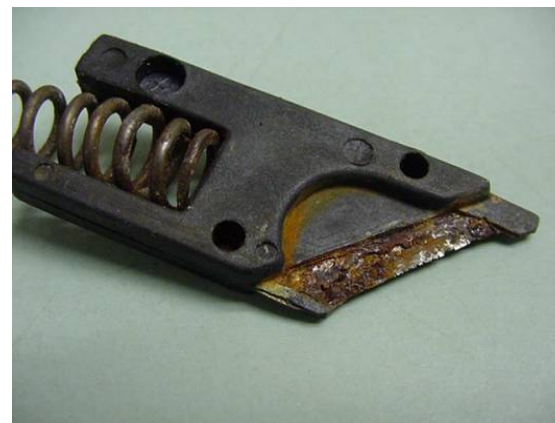
Figure 1.5 - Rusty blade. Source: AMSA.
