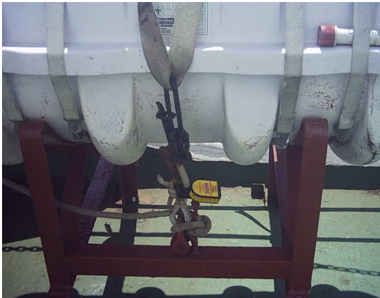
Painter connected to a fixed eye.
