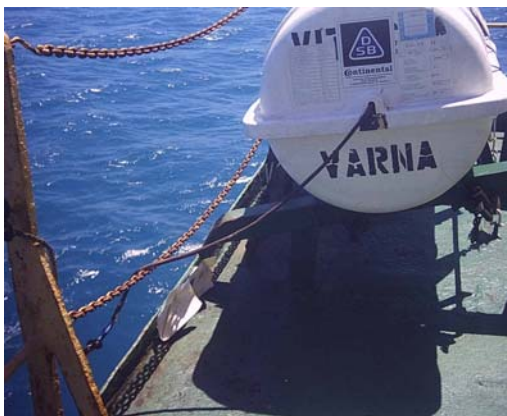
Painter connected to a fix point.
