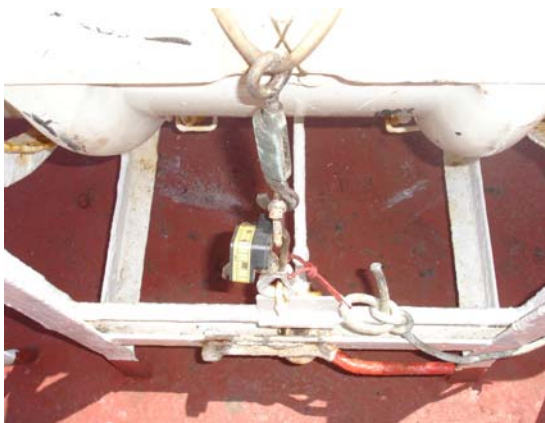
Painter incorrectly connected.
