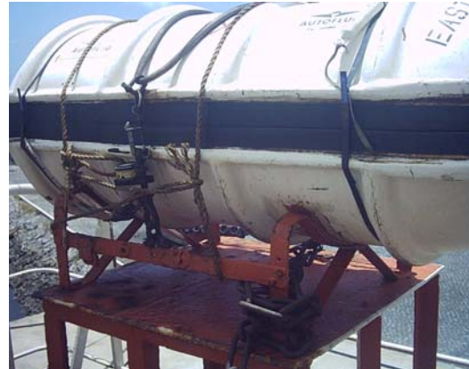
Painter not connected to the HRU.
