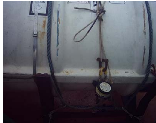
Free-flotation hampered by nylon rope.
