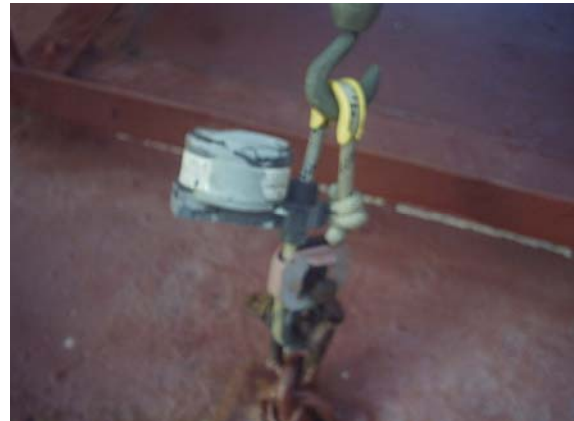
Painter not connected to the HRU.
