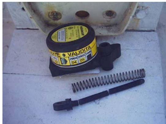
Figure 3.6 - Damaged bolt for EPIRB.
