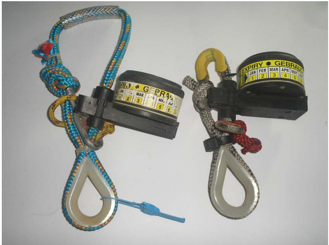
Figure 4.1 - Original unit on the right, manipulated unit on the left.
