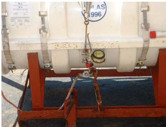
Painter incorrectly connected.
