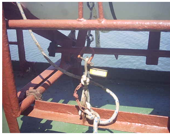
Painter connected directly to weak link.
