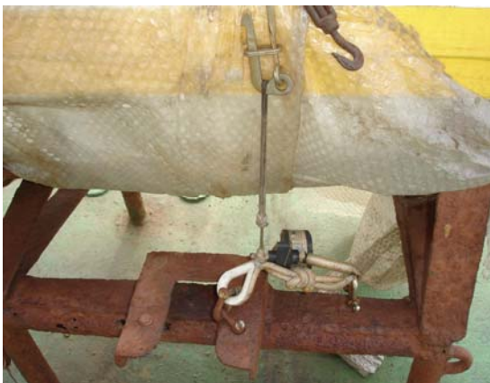
Painter and hook incorrectly connected.
