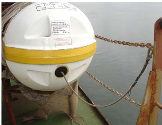
Painter connected to a fix point.
