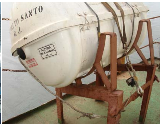
Painter incorrectly connected.
