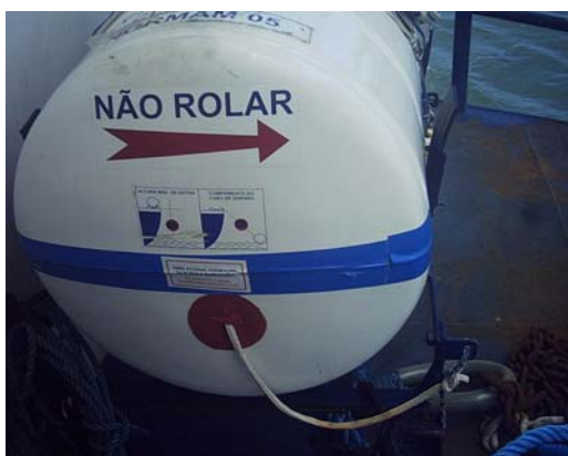
Painter connected to a fix point.
