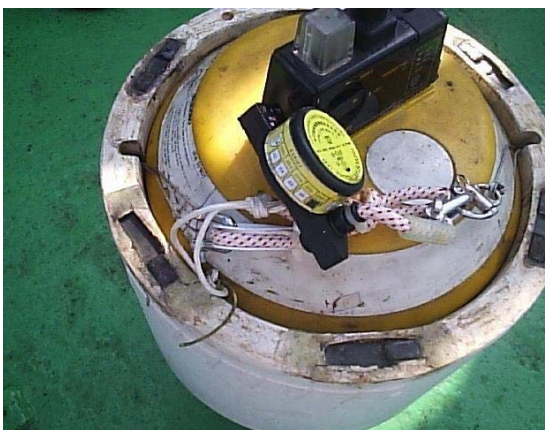
Liferaft HRU used for EPIRB.
