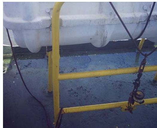
Painter connected to a fix point.
