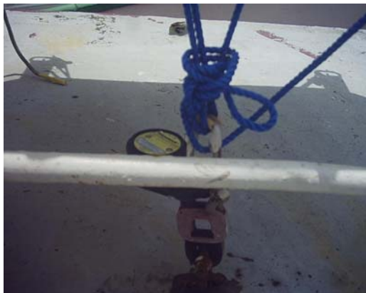
Painter not connected to the weak link.
