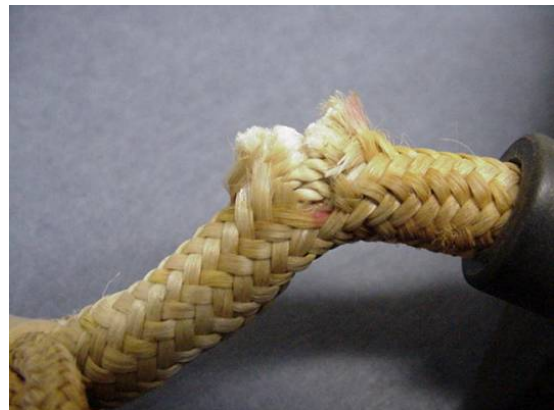
Figure 1.7 - Detail of incomplete cut. Source: AMSA.
