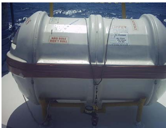
Painter not connected to the weak link.
