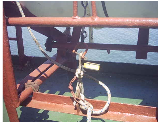
Painter connected directly to weak link.
