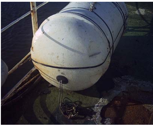
Internal weak link instructions missing.
