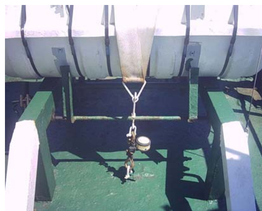
Painter not connected to the HRU.
