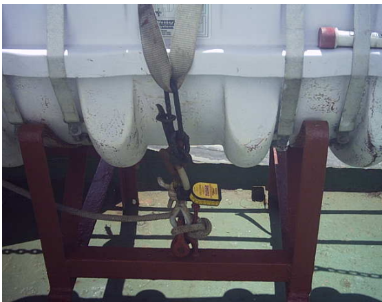
Painter connected to a fixed eye.
