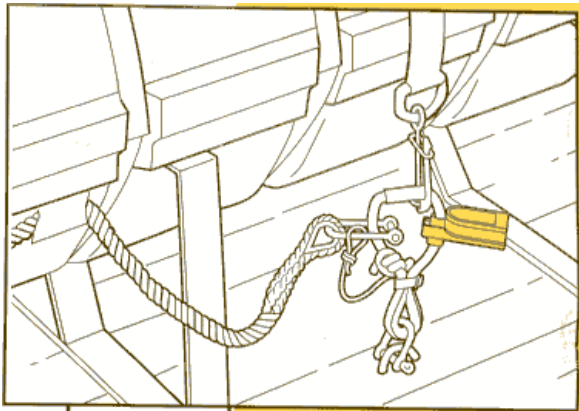
Pains Wessex HRU (pyrotechnic charge) and installation arrangement.
