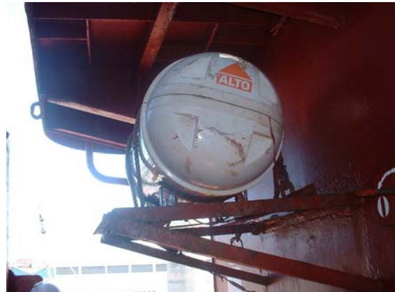
Figure 3.3 - Liferaft stowed 1.7m high. 16
