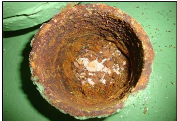
Figure 21: the disinfecting tube blocked by rust.
