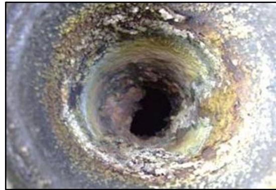
Figure 11: rust status of dosage tube
