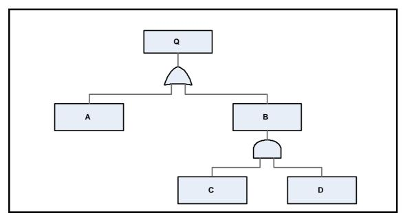
Figure 5.2 – Typical Fault Tree diagram
