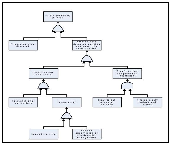
Figure 5.3 – Fault Tree Construction for a security event
