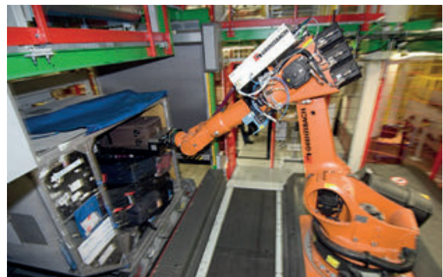
FIGURE 5.2 Manual baggage loading with lift solutions vs. automated baggage loading
