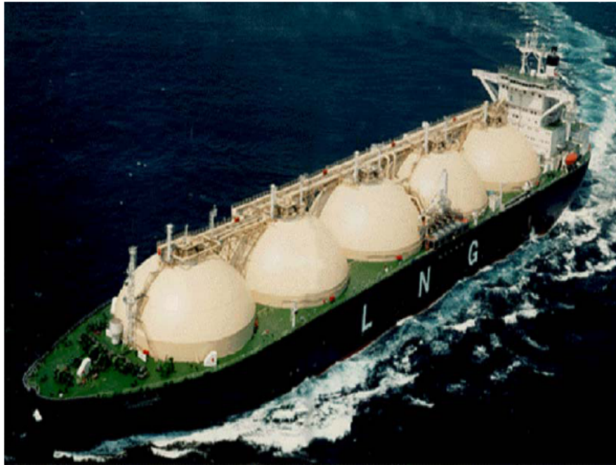
Figure 3- The Appearance of Moss Type LNG Vessels
