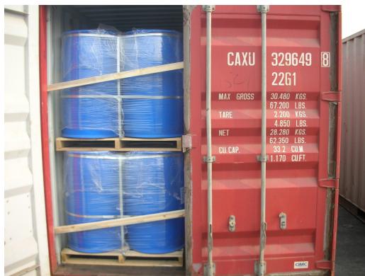
Figure 2.2.3.e The markings on the packaging are not toward the door Resources: Database of TMSA
