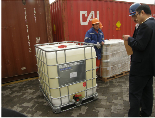
Figure 2.2.3.g The marking of packaging is missing
