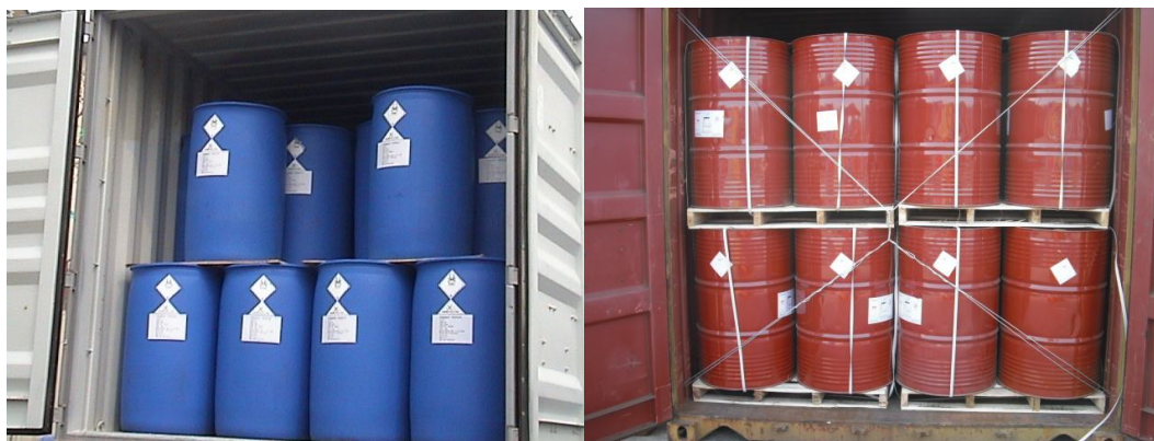
Figure2.2.5.e There is no reinforcing wood for the drums Resources: Database of T MSA
