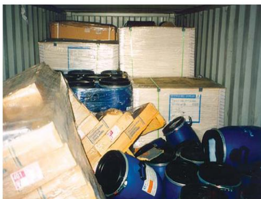
Figure 2.2.5.a Some drums are downwards in the container
