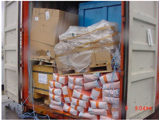
Figure 2.2.5.b The stacking of goods is too random Resources: Database of T MSA
