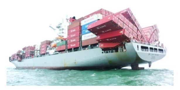
There are several reasons for losses during transport. At sea, it could be causes such as heavy weather, water damage, collision, grounding or fire. For example, the M/V Bai Chay Bridge suffered heavy losses of containers during a category 4 super-typhoon. Several containers were lost overboard or crushed due to the severe rolling experienced by the ship.
