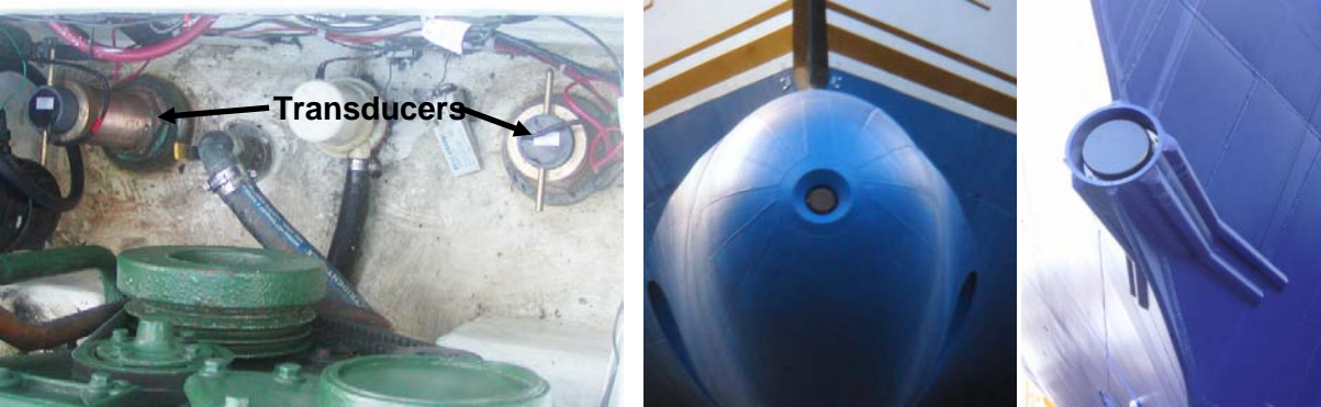
Figure 1: FL-Sonar Transducer Installations (1a. Dual EchoPilot Transducers Mounted Athwartships (left) and b. Single FarSounder Bow-Mounted Transducers (centre and right))
